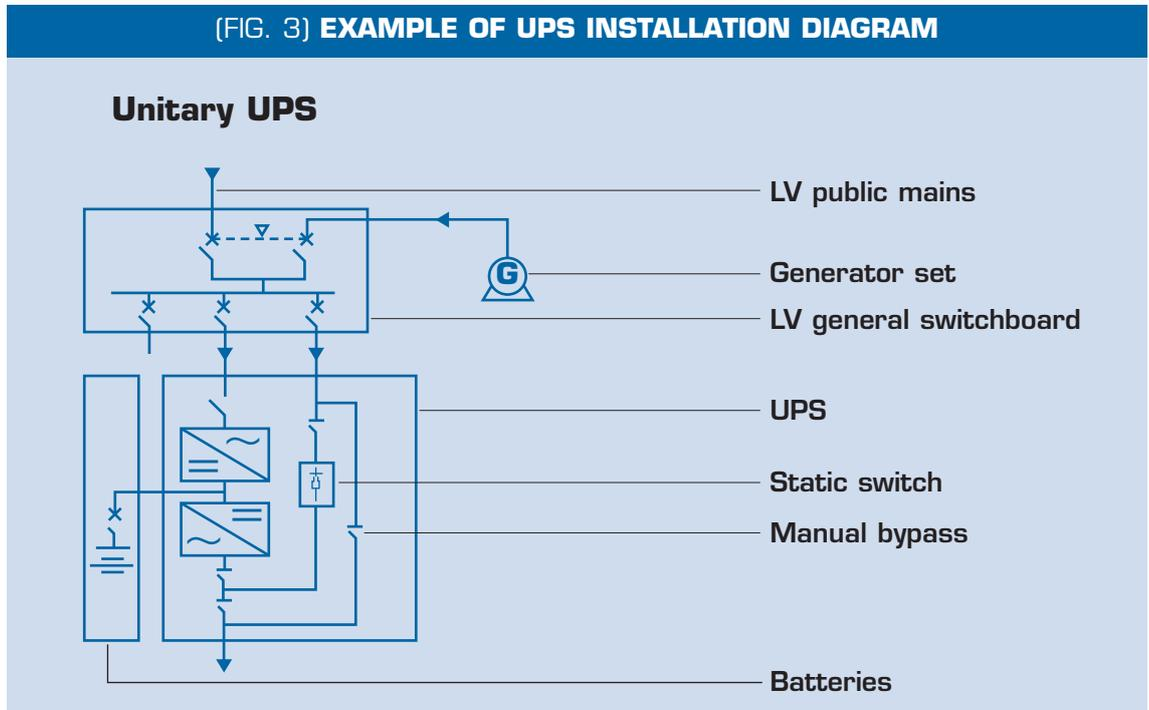
Indeed, in the instance of a very long blackout, it will enable the back-up time provided by the battery to be extended, of course with the battery providing continuity of supply whilst the generator set is starting up and 10 or more minutes of back-up time should it not start up, during which time all the customer application shut-down sequences can be performed.
