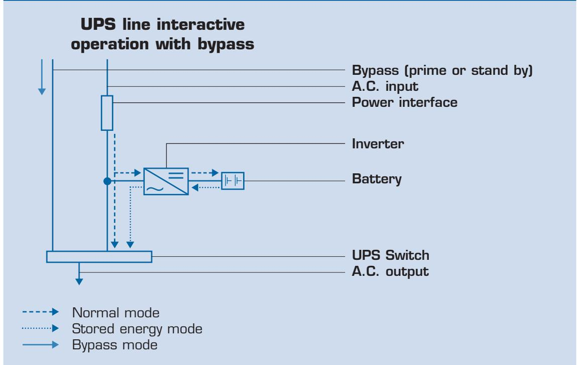
When the a.c. input supply voltage is out of UPS preset tolerances, the inverter and battery maintain continuity of load power in stored energy mode of operation and the switch disconnects the a.c. input supply to prevent backfeed from the inverter.
